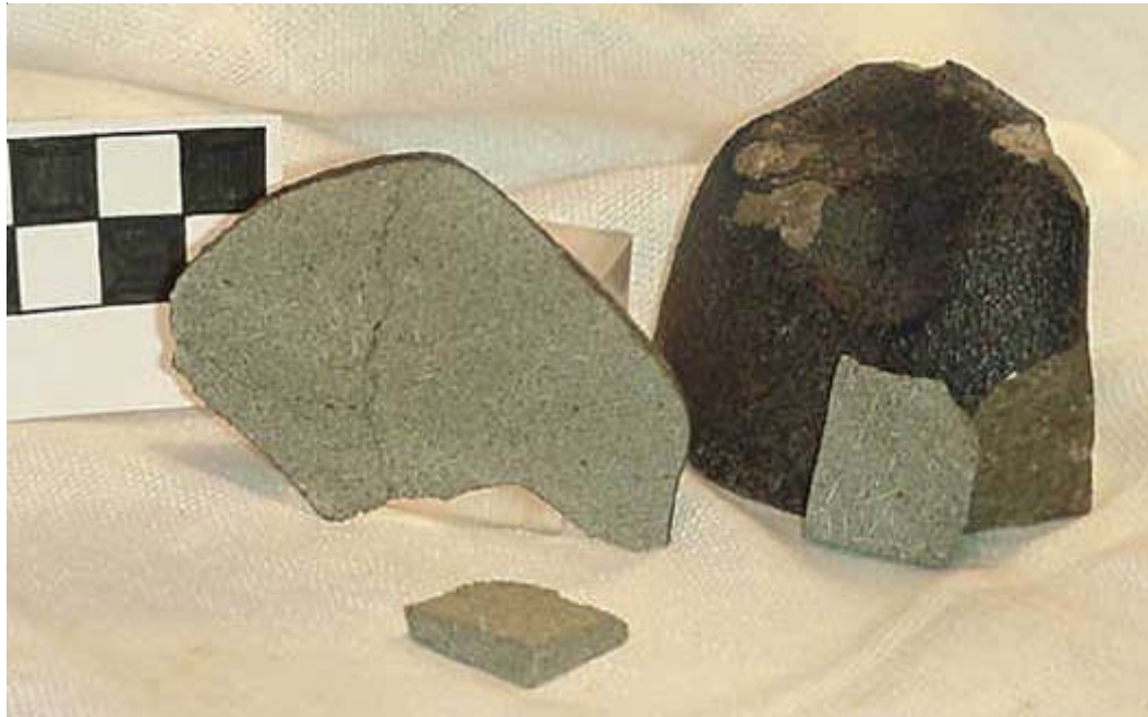
Figure 1: Photograph of NWA 856 (Djel Ibone) kindly provided by Bruno Fectay and Carine Bidaut illustrating thin fusion crust and interior basaltic texture (scale is 1 cm).
